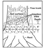
Figure 2. Placement of Shortstop® 2SC as a soil injected treatment
